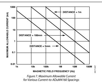
As shown, the ADuM4160 is extremely immune and can be affected only by extremely large currents operated at high frequency very close to the component. For the 1 MHz example noted, a 0.5 kA current would need to be placed 5 mm away from the ADuM4160 to affect the operation of the component.
