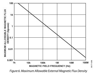
For example, at a magnetic field frequency of 1 MHz, the maximum allowable magnetic field of 0.2 kgauss induces a voltage of 0.25 V at the receiving coil. This is about 50% of the sensing threshold and does not cause a faulty output transition. Similarly, if such an event occurs during a transmitted pulse (and is of the worst-case polarity), it reduces the received pulse from >1.0 V to 0.75 V—still well above the 0.5 V sensing threshold of the decoder.
