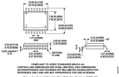
Figure 11. 16-Lead Standard Small Outline Package [SOIC\_W] Wide Body (RW-16) Dimension shown in millimeters and (inches)
