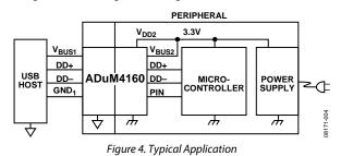
Other than the delayed application of pull-up resistors, the ADuM4160 is transparent to USB traffic, and no modifications to the peripheral design are required to provide isolation. The isolator adds propagation delay to the signals comparable to a hub and cable. Isolated peripherals must be treated as if there were a built-in hub when determining the maximum number of hubs in a data chain.
