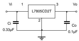
Note: Bypass capacitors are recommended for optimum stability and transient response and should be located as close as possible to the regulators.
