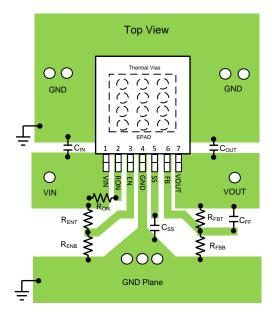
Figure 31. PCB Layout Guide
