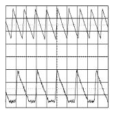
Figure 25. CCM and DCM Operating Modes  $V_{\text{IN}}$  = 24 V,  $V_{\text{O}}$  = 3.3 V,  $I_{\text{O}}$  = 3 A/0.4 A 2  $\mu s/\text{div}$
