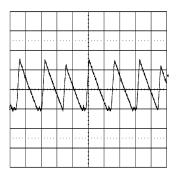
Figure 26. Transition Mode Operation  $V_{IN} = 24 \text{ V}, V_O = 3.3 \text{ V}, I_O = 0.5 \text{ A } 2 \mu\text{s/div}$
