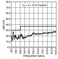
Figure 29. Radiated Emissions (EN 55022 Class B)
