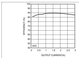
Figure 27. Efficiency  $V_{IN} = 24 \text{ V } V_{OUT} = 5.0 \text{ V}$
