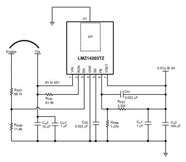
Figure 24. Evaluation Board Schematic Diagram
