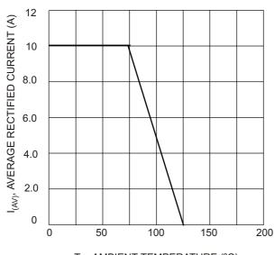
T<sub>A</sub>, AMBIENT TEMPERATURE (°C) Fig. 1 Forward Current Derating Curve
